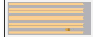
A high-bay shelving system makes maximum use of vertical space. Shelving can be easily adjusted based on book size or box type to condense collections.
