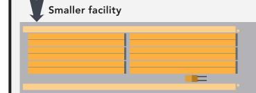
A smaller facility can be built when a high-bay system is compacted to eliminate empty aisle space, which results in decreased operational costs.
