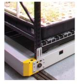
**Carriages**Provide the base of the GROW system to move shelving sections to access individual aisles.
